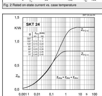
Fig. 4 Transient thermal impedance vs. time
